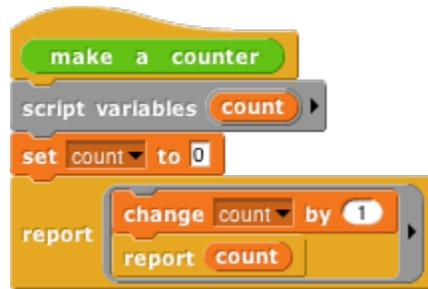
This script implements an object *class*, a type of object, namely the counter class. In this first simplified version there is only one method, so no explicit message passing is necessary. When the **make a counter** block is called, it reports a procedure, the ringed script inside its body. That procedure implements a specific counter object, an *instance* of the counter class. When invoked, a counter instance increases and reports its count variable. Each counter has its own local count:
